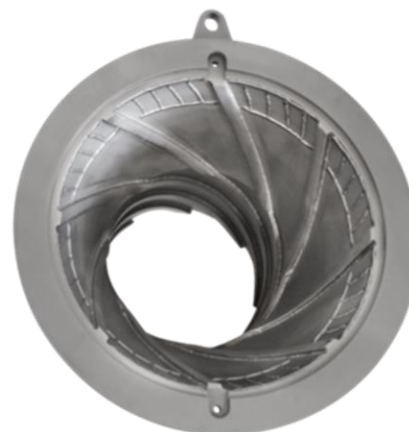
Lining for Simo® grinder refurbished
