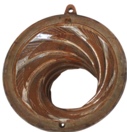
Lining for Simo® grinder before refurbishment
